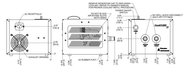
Figure 69. CoolCUBE<sub>II</sub> Circulator
